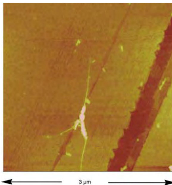
Figure 3. An AFM image of isolated bundles of starch-wrapped SWNTs on a mica surface. Amorphous polysaccharide material is seen to aggregate with the nanotubes mostly at junctions between bundles.
