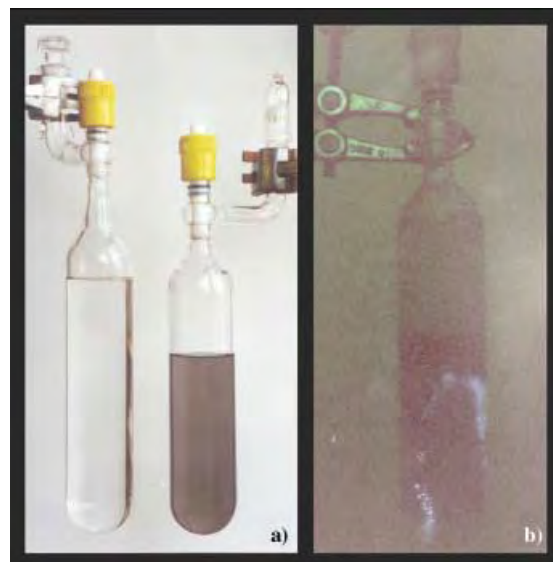
Figure 1. a) Two samples of GaEt 3 . Left: a pure sample; Right: a sample after 15 freeze–thaw cycles under argon, b) the triboluminescence flashes which occur upon warming a sample of GaEt 3 under argon that had been frozen in liquid nitrogen.
